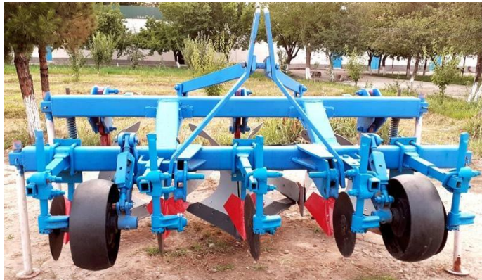
Fig.4. Experimental model of a frontal plow with a corner-mounted plow
