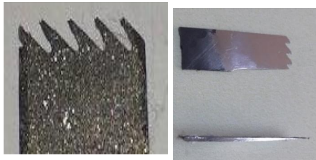
Fig. 6. Special samples - microsections cut from linter saws with preparation of the controlled surface in the form of an oblique cut
