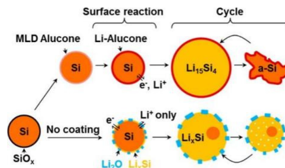
Figure 13 Schematic of surface reactions and cycle behaviors of silicon nanoparticles with different coating conditions and captured in situ TEM images of the alucone-coated Si nanoparticles during the lithiation/delithiation behaviour. Copyright 2014 ACS Nano
