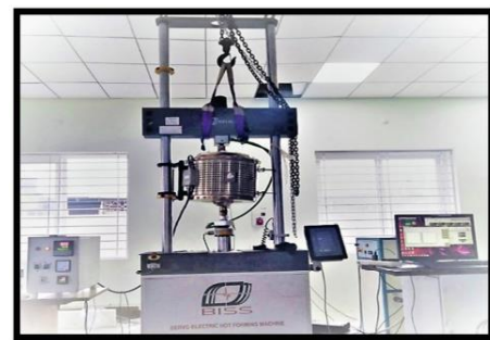
Figure 2 : Uniaxial Tensile Test Machine
