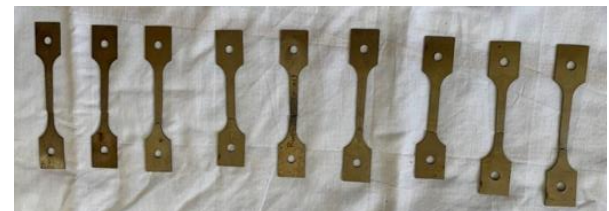
Figure 3 : Uniaxial Tensile Test Specimens in all orientation
