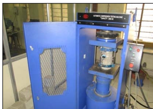
Fig.1.: Test setup for stress-strain measurements
