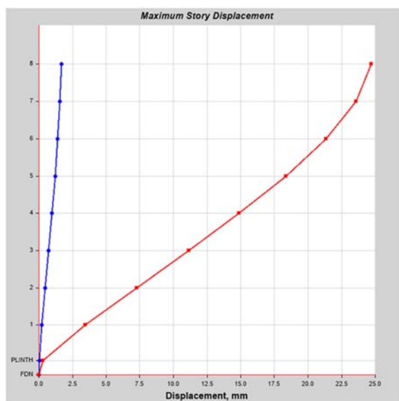
Figure-4: EQY Storey Displacements C-230x600 (C40 25)
