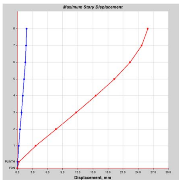
Figure-6: EQY Storey Displacements C-230x525 (C-50 25)
