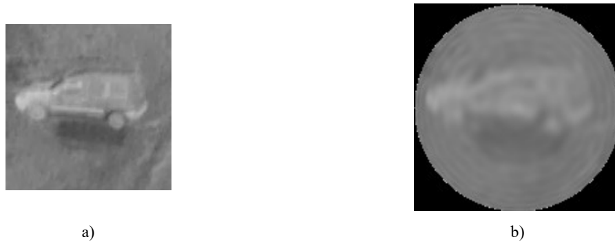
Fig. 2. Restoration of a thermal image of imperfect quality using ZM: a) - the original image; b) - the restored image at n = 40
