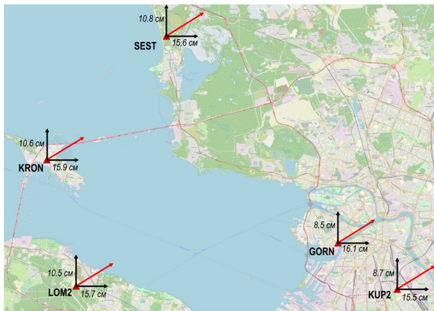
Fig. 10. The sketch-map of the location of the studied stations and their movements
