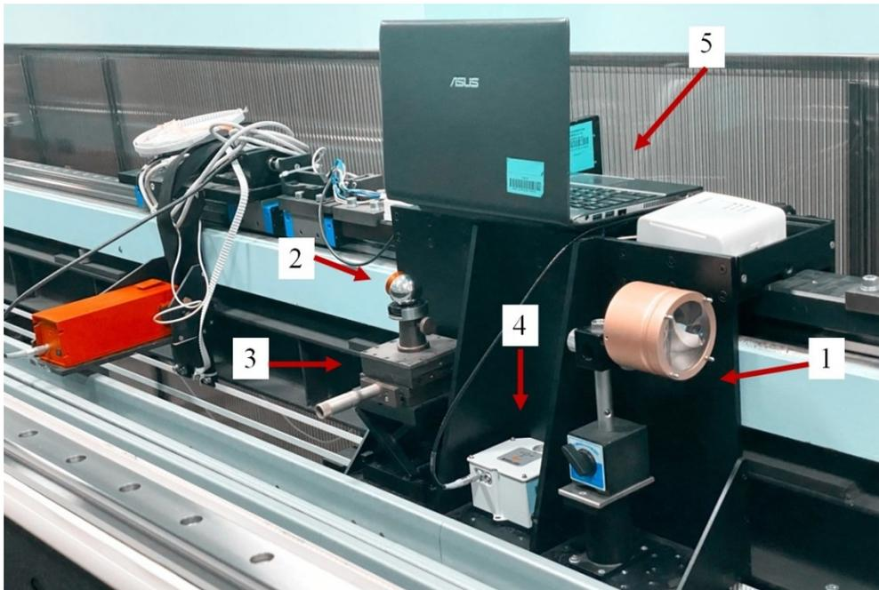
**Fig. 4.** The composition of the mobile platform. 1 - corner reflector of the interferometric system, 2 - corner reflector of the absolute tracker, 3 - adjustable turntable, 4 - Leica Nivel inclinometer, 5- PC for controlling the equipment of the moving platform.
