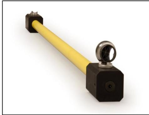
**Fig. 1.** Measure for verification of laser coordinate measuring systems.
