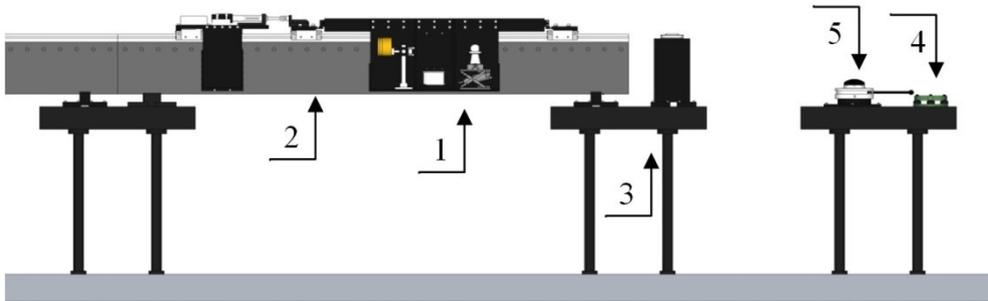
**Fig. 3.** Layout diagram of the stand. 1 - movable platform, 2 - rolling rail, 3 - optical table, 4 - slot for absolute trackers like Leica AT401-AT403; 5 - slot for absolute trackers like Faro Laser Tracker, Leica AT960 - AT930.
