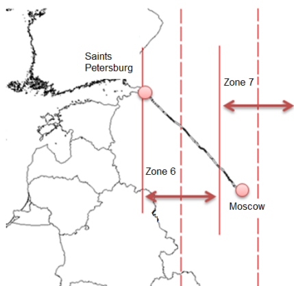
Fig. 1. The layout of the object relative to the 6-degree zones SK-42 (SK-42 is the state system of geodetic coordinates based on the Krasovsky reference ellipsoid).
