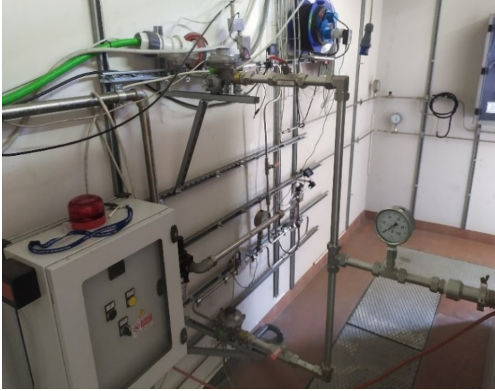
Fig. 2. Section 1 of the apparatus with the lines of air and technical gases as well as reference thermal mass flow meters and pressure regulators.
