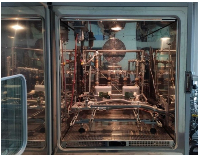
Fig. 3. Section 2 of the apparatus and the climatic chamber to control the testing conditions.
