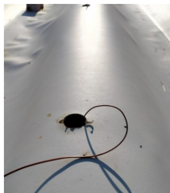
Fig. 5. Thermocouple buried into the soil at 0.10 m below the ground in the mulched field section.
