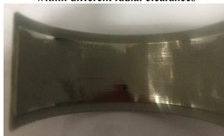
Fig. 11 Wear in bearing bush
