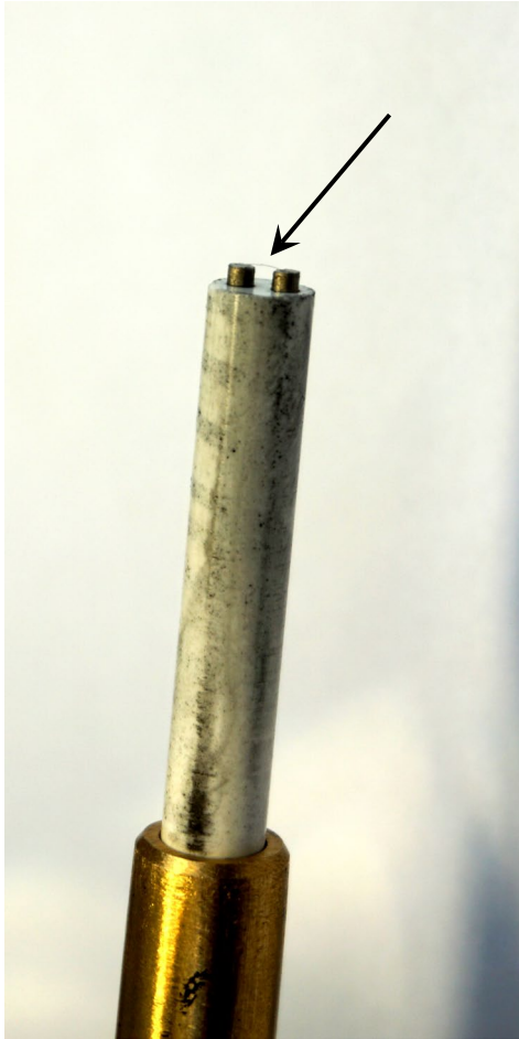
Fig. 4: Photograph of the tip of a fine-wire thermocouple probe deployed to capture gas temperature profiles in the appendix gap
