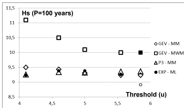
Fig. 3. Variation of the hundred-year return period waves for different forecasting models depending on thresholds in the point in Mohammedia's coast
