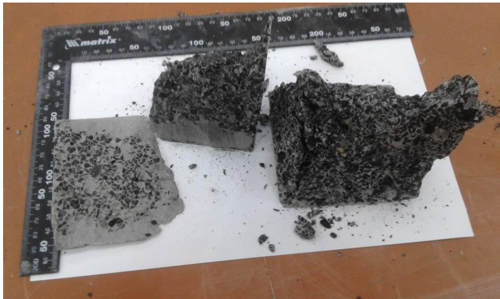
Fig. 3. Sample segregation under compressive strength testing
