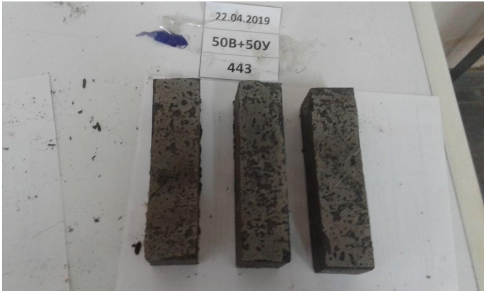
Fig. 1. The samples made from UGM-70 binder mixture and a fine fraction of coal in a 50/50 ratio
