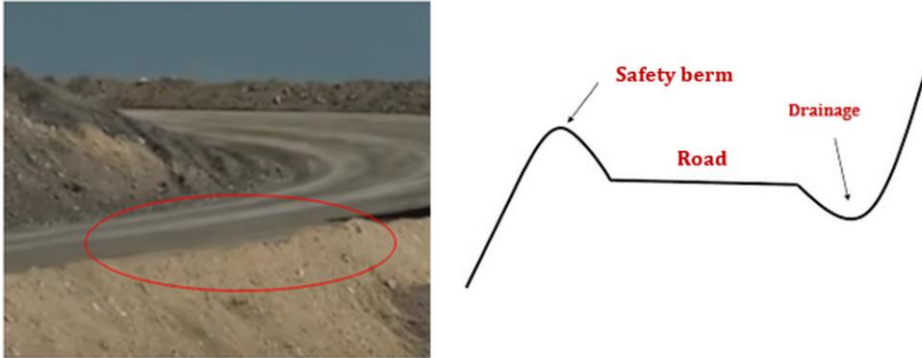
Fig. 11. Scheme of safety berms and drainage
