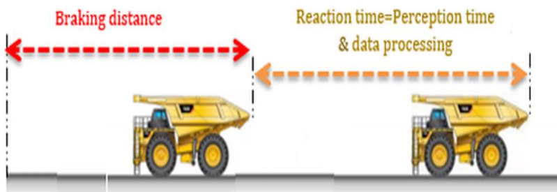
Fig. 4. Braking distance of autonomous truck
