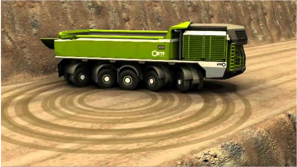
Fig. 5. General view of a dump truck with five driving axles and synchronously turning wheels to minimize the width of the turn area
