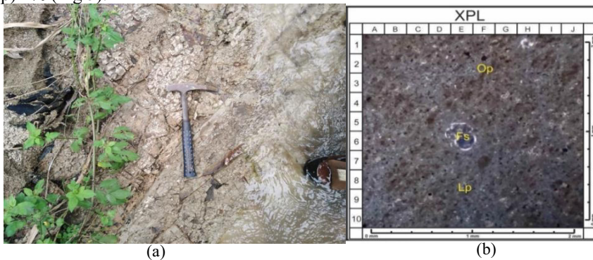
Fig. 5. (a) Claystone unit at STA 11 (b) Petrographic appearance (opaque minerals (Op), clay minerals (Lp), foraminifera fossils (Fs)).
