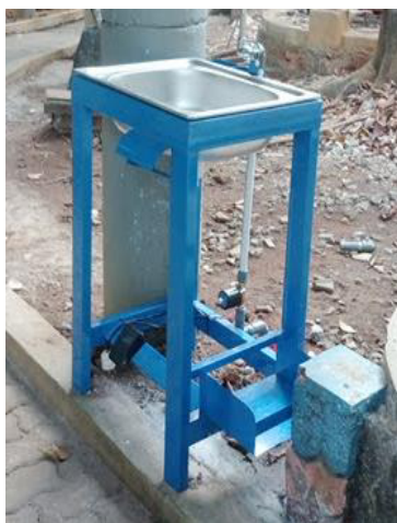
Fig. 2. Ablution tap design (knee activation).
