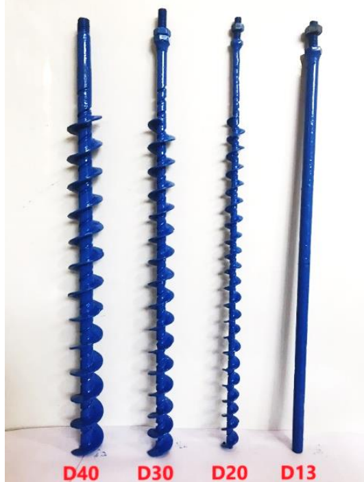
Figure 1. Model piles used in tests.
