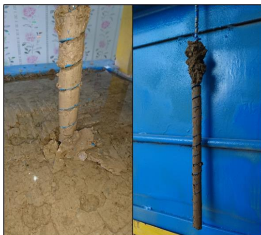
Figure 7. The cylindrical shear failure mode of screw pile.
