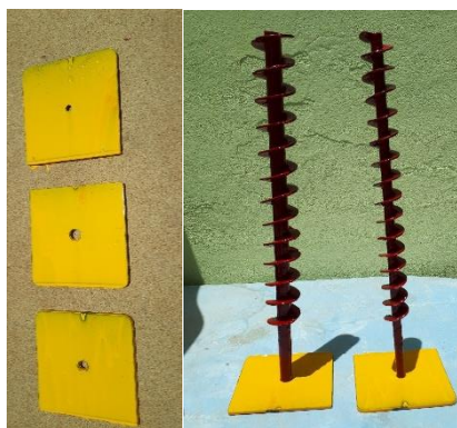
Figure 4. Cap of screw pile (120×120×6 mm). Figure 5. Insertion and adjustment of screw pile.
