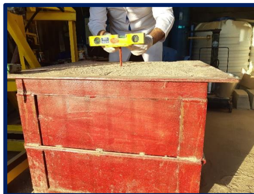
Figure 4. Cap of screw pile (120×120×6 mm). Figure 5. Insertion and adjustment of screw pile.
