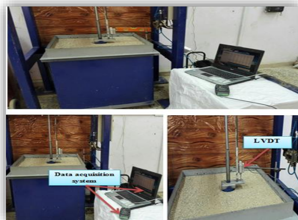
Figure 9. Linear variable differential transformer (LVDT).
