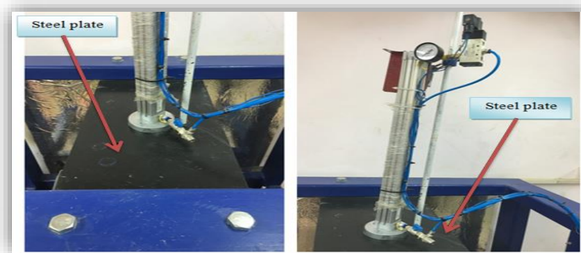
Figure 5. Steel plate for supporting a jack.
