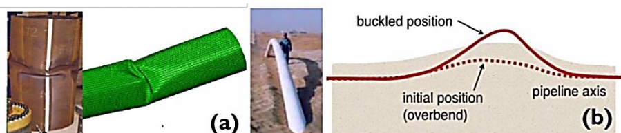
Figure 3. (a) Excessive pipe wall compression causes local when the pipe is bent longitudinally and (b) Excessive axial loading causes buckling beam for buried pipeline [22].
