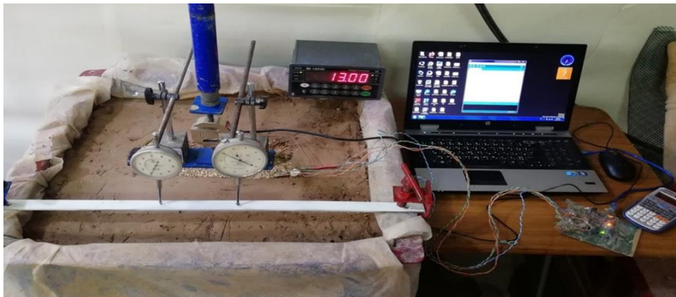
Figure 1. Soil model apparatus.
