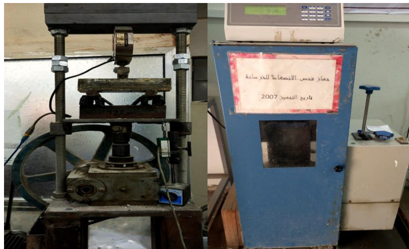
a) Compressive strength device b) Flexural strength device Figure 2. Mechanical test machines.
