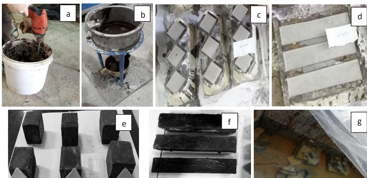
Figure 1. Grouts and samples preparation: a) mixing, b) fluidity test, c) cubs casting, d) prisms casting, e) cubes demolded, f) prism demolded, and g) curing.
