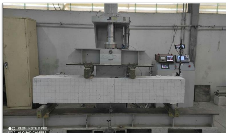
Figure 3. Position of beams in the load-testing machine.
