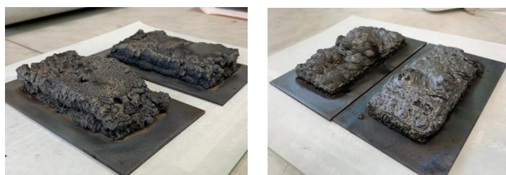
Fig. 5. View of the samples after annealing in a furnace
