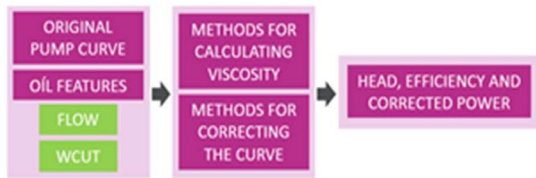
Fig. 5. Process of correction of the curve of the pump
