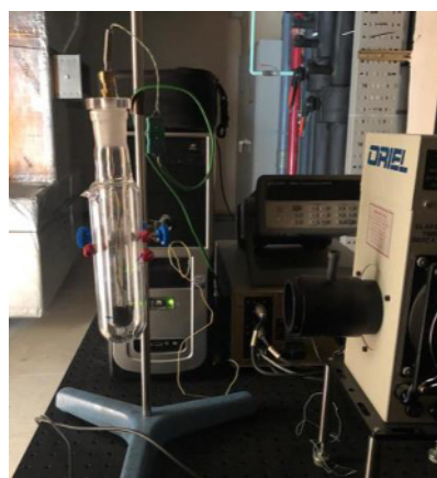
Fig. 1. Experimental setup for the measurement of temperature increase of optically excited nanofluids.
