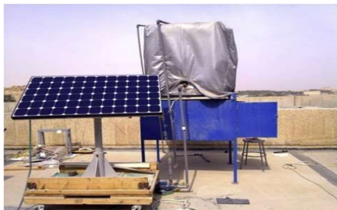
Fig. 11. Experimental setup for cooling the PV module [45]
