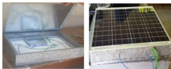
Fig. 8. a) PCM box b) PV-PCM connection [42]
