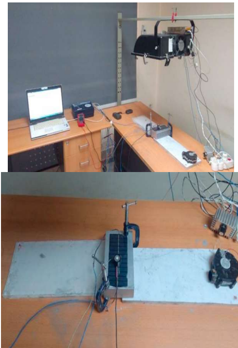
Fig. 15. The indoor experimental setup for heat sink cooling[48]
