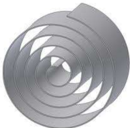
Fig. 2. Air turbulator used to improve the HE-1 heat exchanger operation in the conditions of a non-uniform flow of mediums [13]
