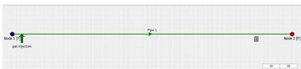
Fig. 5. Model of the oil transport system used in the simulator, oil flow direction from the underwater head (Node 1) to the platform (Node 2).
