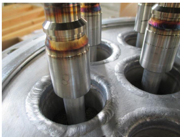
Fig. 2. Tube sheet of the molten salt heated steam reformer with catalyst and membranes in the inner tubes developed in the project CoMETHy [4].
