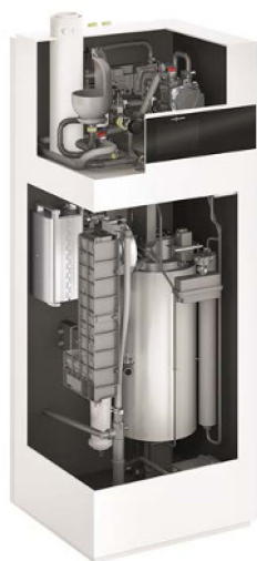
Fig. 6. Vitovalor PT 2 based on PEM-LT technology P_{el} : 750 W, P_{th} : 1,1 kW th P_{th} from gas boiler: individual scalable from 11,4 kW, 24,5 kW to 30,8 kW Hot water storage tank: 220 l
