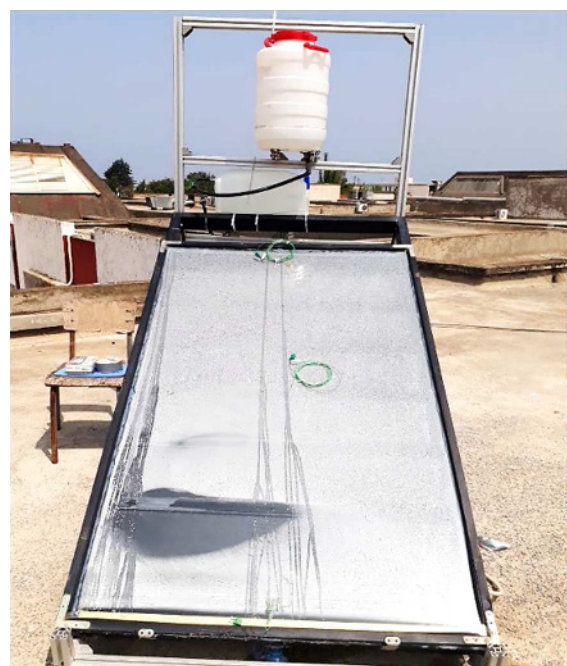
Fig. 2. Experimental set up of novel cascade solar still [9].
