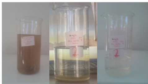
Fig.5. Depicts the effects of (alum coagulant dose :150 mg/L and pH at 7) on domestic wastewater effluent (before and after
