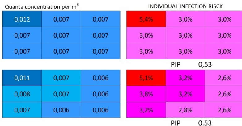
Fig. 3 - Total air system quanta concentration, individual and collective infection risk with infected person in sector 1, the one at the top left. Return air intake in top left sector above and in bottom right sector below
