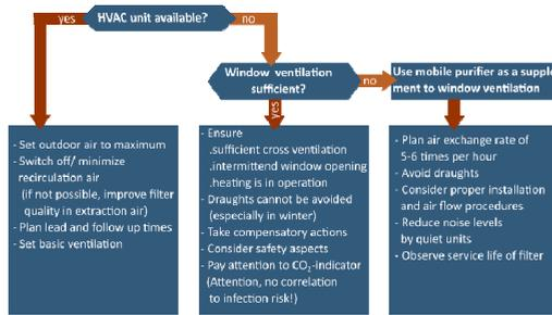
Fig. 1. Matrix to decide on different ventilation measures.
