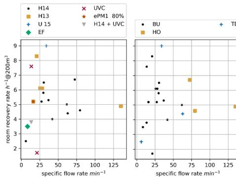
**Fig. 11.** Recovery rate for a room of 200 m<sup>3</sup> and 6 h<sup>-1</sup> vs. specific flow rate with filtration principle and flow direction as parameter.
