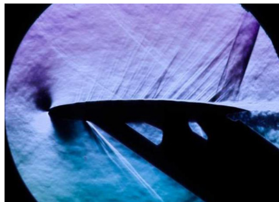
Fig. 10. Schlieren picture taken at M_1 = 0.988 showing flow disturbances on the upper surface of the airfoil due to imperfect coverage of leadwires
