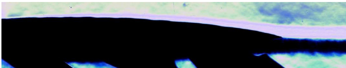
Fig. 18. Schlieren visualization of the upper surface boundary layer in case with rough leading edge. ( M_1 = 0.76 )
