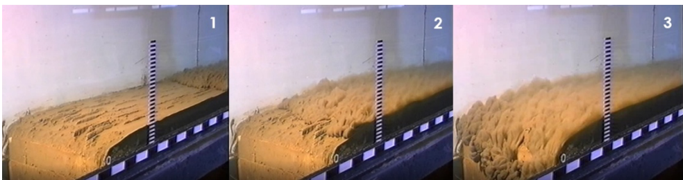
Fig. 9. Demonstration of density currents after water injection in laboratory.
