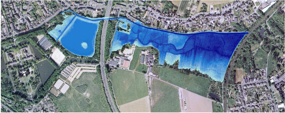
Fig. 5. Maximum reservoir area by the maximum reservoir level (+3,37 m / 57,10 masl).
