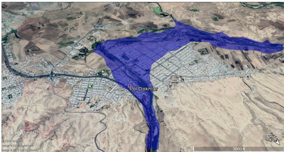
Fig. 9. Satellite image of the flooding extent in the PolDokhtar city located in the downstream of the unconstructed Tang-e-Mashoureh reservoir.
