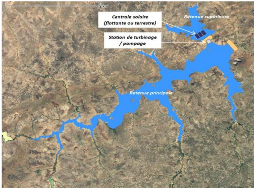
Fig. 7. PSP implementation for Bassiéri Dam.
