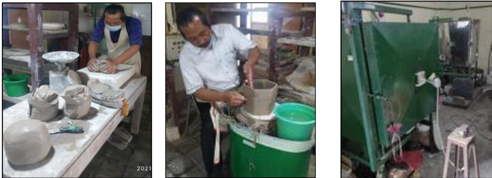
Fig.1. Wedging process (left), hand-building technique (center), and firing process (right).
