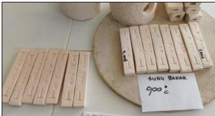
Fig. 5. Test pieces of ceramic, fired at 900°C temperature.
