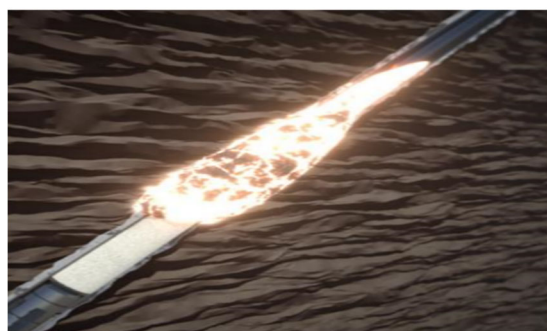
Figure 2. Schematic diagram of the thermite P&A technology(right)
