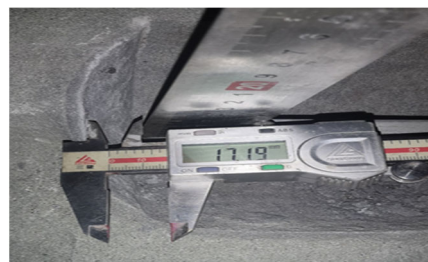
Figure. 6 The diameter and height of the hole before and after the closed environment
