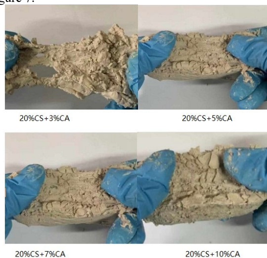
Fig. 5 Curing effect of crosslinked bonding and crystalline curing compound working fluid
