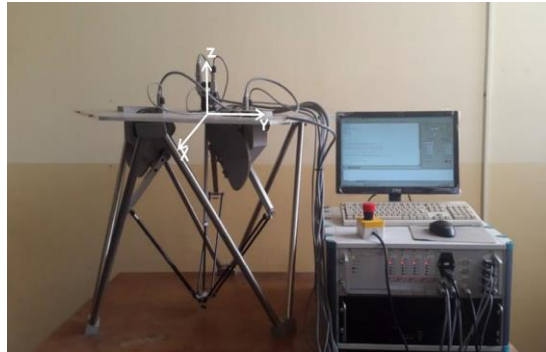
Fig. 4. Delta robot experimental platform
