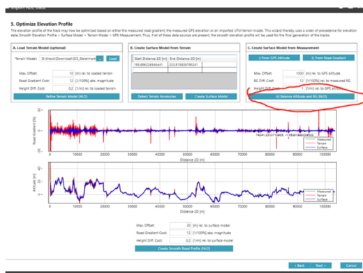
Figure 4 Schematic diagram of slope calculation and correction based on AVL VSMTM
