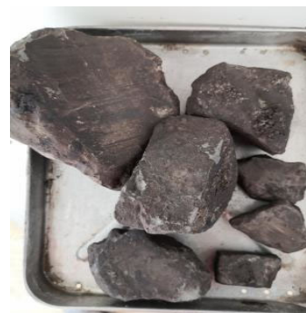
Fig. 10 The cement block returned after the first cement injection in Zhong-14 well
